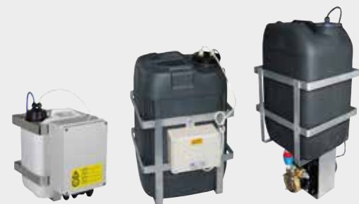
WASPT WASHER PUMP AND 5 OR 23 LITER TANK • Polyethylene tank with stainless steel cage • Delivery head: 5m (16ft), 11m (36ft) or 30m (98ft) • Versions with alarm for the lack of liquid in the tank • Operating temperature: from -10°C (14°F) up to +60°C (140°F) • Available voltages: 230Vac, 120Vac, 24Vac
