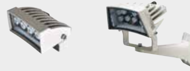
GEKO IRN AND GEKO IRH LED ILLUMINATOR • High efficiency ultimate SMD LED technology • High efficiency heat sink body to ensure maximum LEDs durability • Strong aluminium structure • Supply voltage: 12Vdc, 24Vdc, 24Vac or from 100Vac up to 240Vac • Beam patterns: 10°, 30°, 60° • Adjustable built-in photocell • Supplied with a wall-mount bracket • IP66/IP67
