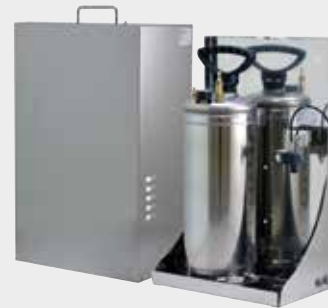
WASNX WASHER PUMP WITH SOLENOID VALVE FOR STAINLESS STEEL PRODUCTS • Enclosure made of stainless steel AISI 316L • Delivery head: up to 30m (98ft) • Water tank capacity: 10l (2.6gal) • Operating temperature from -20°C (-4°F) up to +60°C (140°F) • Available voltages: 230Vac, 120Vac, 24Vac
