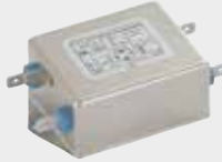
FM1010 EMC FILTER FOR MARINE CERTIFICATION • The filter must be connected to the power line of the equipment • The filter is not explosion-proof certified • Implement adequate protection if used in potentially explosive classified environments (e.g. Atex) • Electrical data: from 0 up to 250V DC/AC 50/60 Hz, 6A
