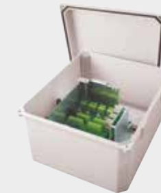
COMB COMMUNICATION BOX IN POLYCARBONATE • Designed to work exclusively with Videotec products and accessories • 1 SFP port, MSA compliant, Fast Ethernet (100BASE-FX), for fiber optic connection (splice tray included in the product) • 3 RJ45 ports, Fast Ethernet (10BASE-T/100BASE-T) • 2 bypass for analog video signals with BNC connectors and 2 bypass for I/O signals with multi-pin connectors • Extended/Industrial range electronics
