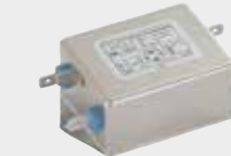
FM1010 EMC FILTER FOR MARINE CERTIFICATION • The filter must be connected to the power line of the equipment • The filter is not explosion-proof certified • Implement adequate protection if used in potentially explosive classified environments (e.g. Atex) • Electrical data: from 0 up to 250V DC/AC 50/60 Hz, 6A
