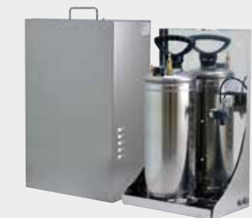
WASNX WASHER PUMP WITH SOLENOID VALVE FOR STAINLESS STEEL PRODUCTS • Enclosure made of stainless steel AISI 316L • Delivery head: up to 30m (98ft) • Water tank capacity: 10l (2.6gal) • Suitable for Videotec products • Operating temperature from -20°C (-4°F) up to +60°C (140°F) • Available voltages: 230Vac, 120Vac, 24Vac
