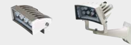
GEKO IRN AND GEKO IRH LED ILLUMINATOR • High efficiency ultimate SMD LED technology • High efficiency heat sink body to ensure maximum LEDs durability • Strong aluminium structure • Supply voltage: 12Vdc, 24Vdc, 24Vac or from 100Vac up to 240Vac • Beam patterns: 10°, 30°, 60° • Adjustable built-in photocell • Supplied with a wall-mount bracket • IP66/IP67
