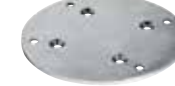
NXPTZTW PARAPET OR CEILING MOUNTING BRACKET • AISI 316L electropolished stainless steel • Load rating: 40kg (88lb) • Dimensions: Ø 238mm (9.4in)
