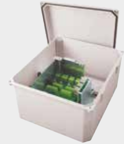
COMB COMMUNICATION BOX IN POLYCARBONATE • Designed to work exclusively with Videotec products and accessories • 1 SFP port, MSA compliant, Fast Ethernet (100BASE-FX), for fiber optic connection (splice tray included in the product) • 3 RJ45 ports, Fast Ethernet (10BASE-T/100BASE-T) • 2 bypass for analog video signals with BNC connectors and 2 bypass for I/O signals with multi-pin connectors • Extended/Industrial range electronics
