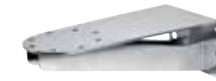
NXPTZWB WALL MOUNT BRACKET • AISI 316L electropolished stainless steel • Load rating: 40kg (88lb) • Length: 400mm (15.7in) • Can be coupled with modular components (NXPTZCW, NXPTZCOL)
