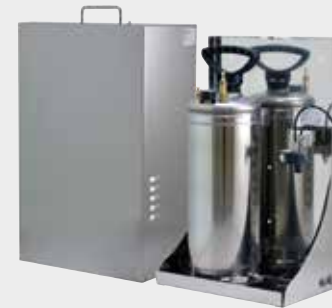
WASNX WASHER PUMP WITH SOLENOID VALVE FOR STAINLESS STEEL PRODUCTS • Enclosure made of stainless steel AISI 316L • Delivery head: up to 20m (66ft) • Water tank capacity: 10l (2.6gal) • Operating temperature from -20°C (-4°F) up to +60°C (140°F) • Available voltages: 230Vac, 120Vac, 24Vac
