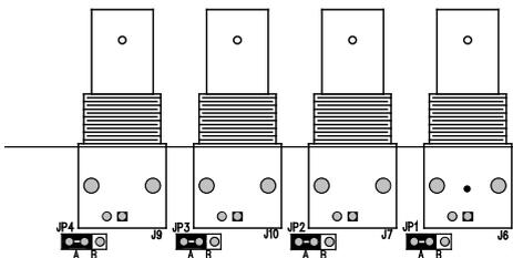
Example: all input with 75 Ohm load inserted
