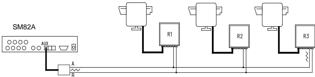
Receivers R1, R2 should not have the termination resistance inserted. The maximum length of the line, from end to end (from the matrix AUX line to receiver R3), is 1200 metres.
