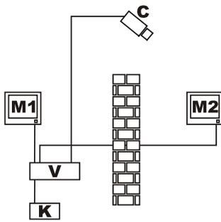
In this example M1 is the *master monitor*, M2 the *public monitor*. Fixed camera C frames the public monitor.
