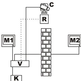
In this example M1 is the *master monitor*, M2 the *public monitor*. Pan & tilt camera C frames the public monitor.
